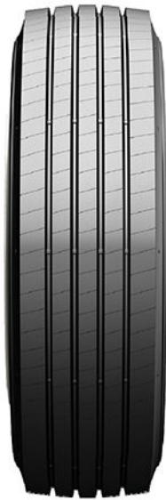
FIG. 1 Front View of the 245/70R19.5 136/134M Radial Truck Standard Reference Test Tire SW
