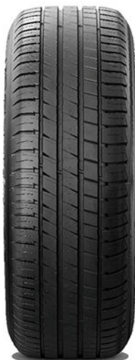
FIG. 1 Front View of the 225/45R17 94V XL Radial Standard Reference Test Tire
