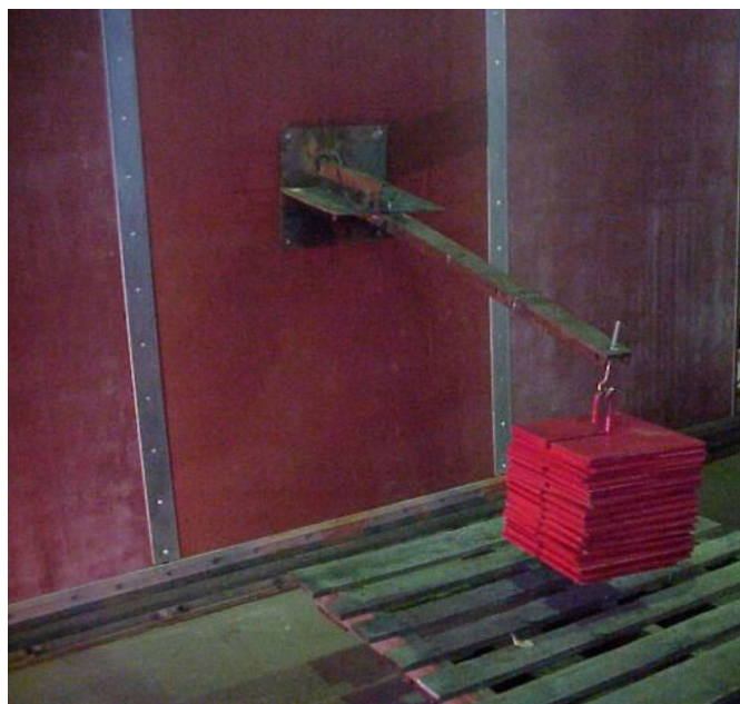
FIG. 2 Loading Bracket with Load Applied at 915 mm [36 in.]
