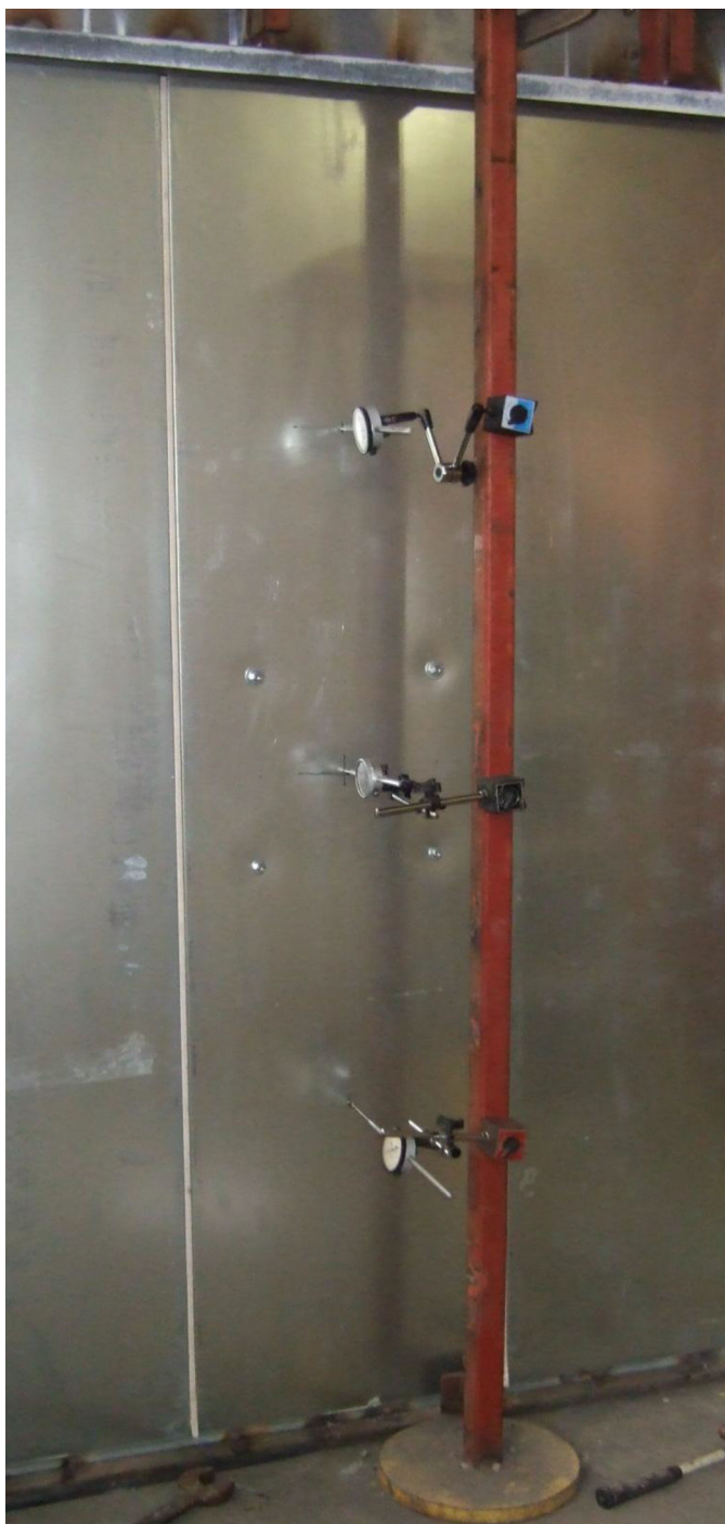
FIG. 1 Setup to Measure Deflection
