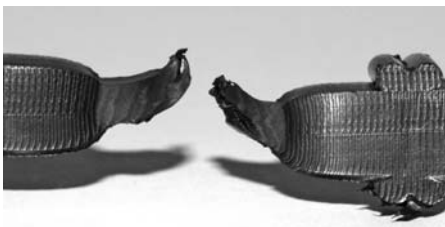
FIG. 2 Ductile Rupture Outside Fusion Interface
