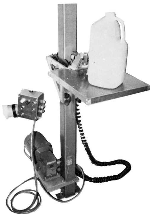
FIG. 1 Apparatus for Dropping Containers
