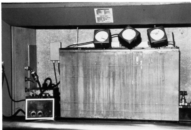
FIG. 1 Rotating Vessel Oxidation Test Apparatus
