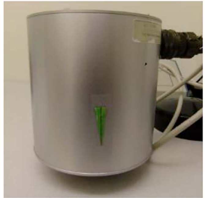
FIG. 2 Vertical Indicator Arrow Affixed to Side of Portable Reflectometer
