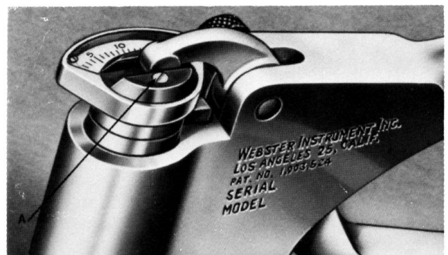
FIG. 3 Zero Adjustment Screw, A (indicated by arrow)
